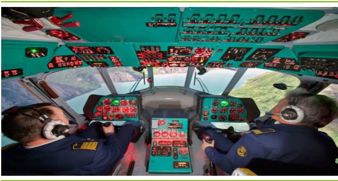
Figure 7. Mi-8 attack helicopter combat training simulator
