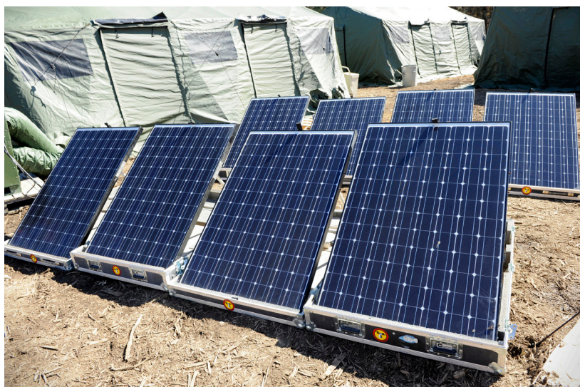
To provide power to Marines in the field, the Office of Naval Research developed this 300-watt photovoltaic battery system, known as the Ground Renewable Expeditionary Energy System (GREENS). Courtesy of U.S. Navy, photo by John F. Williams.
